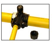
Line marked for stab depth should be no more than 3/4" from face of compression nut.
