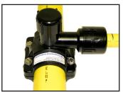
16 through allow service, back punch up until the top of the punch is flush with top of saddle. It is important that the punch does not protrude above the top of the saddle tee.
